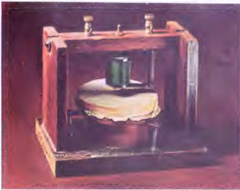
On June 3, 1875, Alexander Graham Bell first transmitted recognizable voice sounds on this ingenious instrument. It employed a tightly stretched membrane, called "goldbeater's skin," which was sensitive to sound waves.
